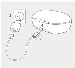
Plug the larger end of the charging cable into the power supply.
